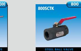
Reduced bore Threaded ends Body Material: A105 Size: 1/4~2
